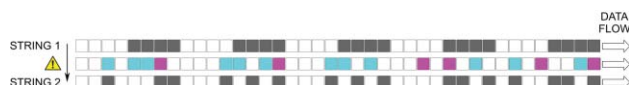
Fig. 7 Schematic representation of modulating a string of digits in Type II hybrid systems. The triangle denotes the appearance of data reading error.
